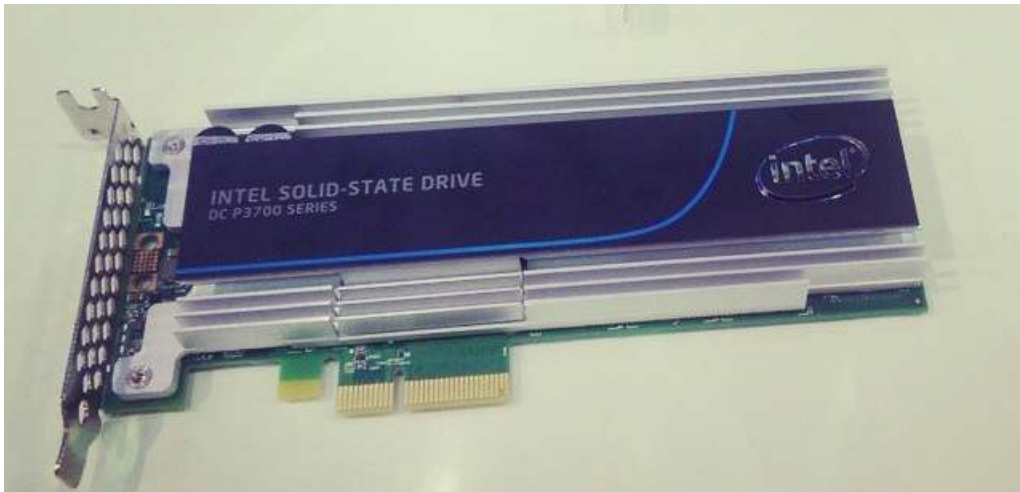
FIGURE 2: An Intel enterprise-grade PCIe drive. They are quite large and require more than twice the space of a typical SATA SSD.
